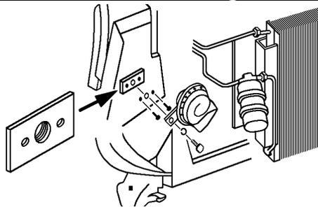
66-67 Horn Mounting Plate on the Fender Skirt
