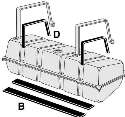
**Fuel Tank Strap Mounting Anti-Squeak Pads**
