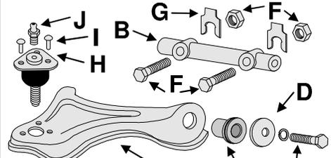
D Upper Control Arm Bushing Concave Steel Retainer
