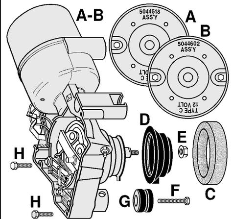
**68-82 Rebuilt Wiper Motors**
